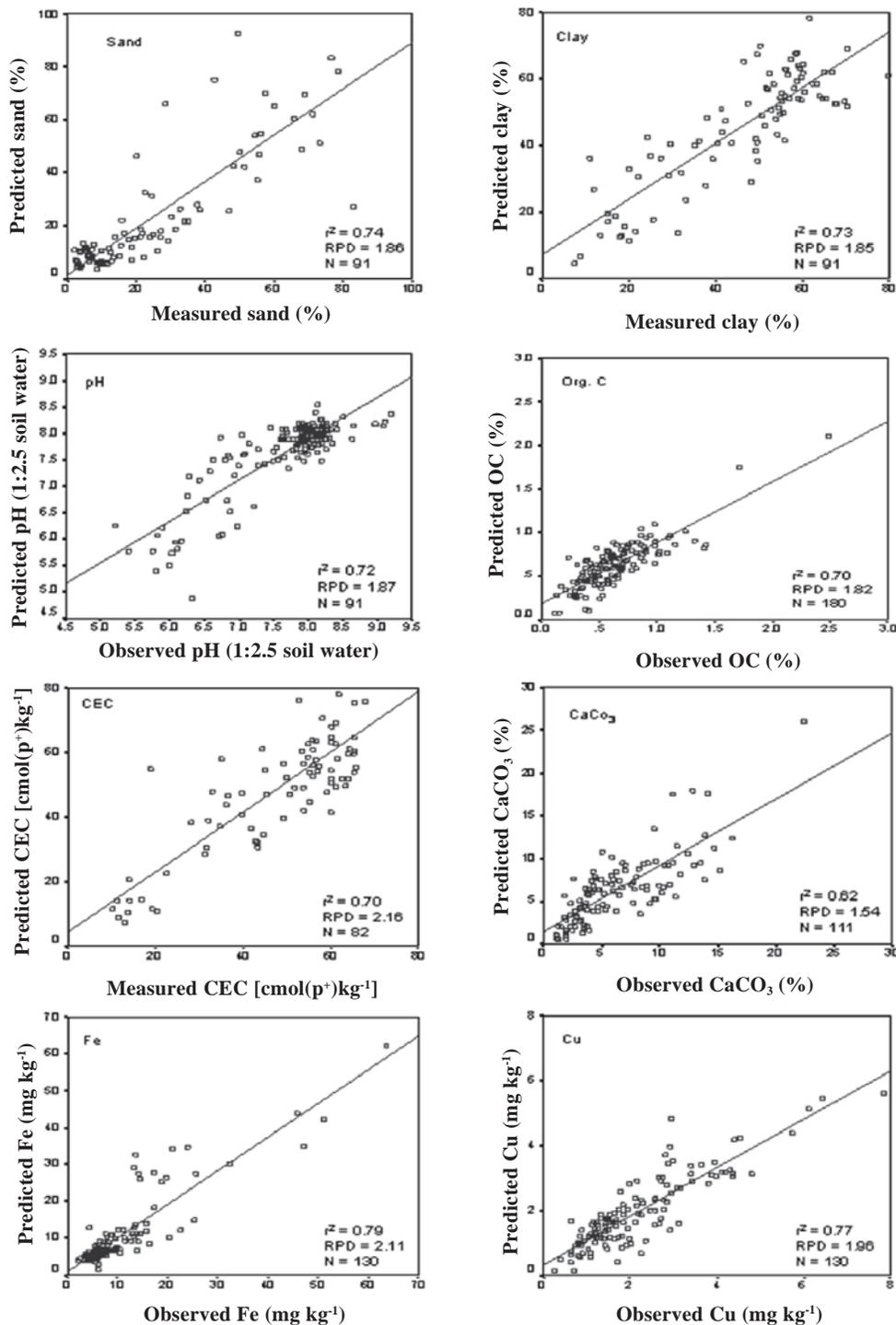
Fig. 3. Scatter plots of observed and predicted values of different soil properties in the validation datasets
