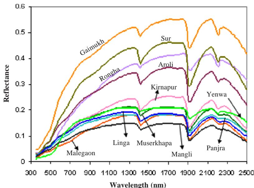
Fig. 2. Reflectance spectra of surface soils of selected soil series of Nagpur District
