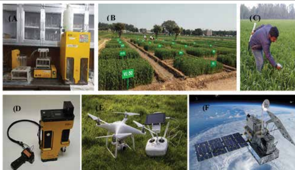
Figure 2. Techniques for canopy N content estimation: (A) Traditional laboratory-based N estimation (Kjeldahl apparatus), (B) Field experimentation for N management, (C) Chlorophyll (SPAD) meter, (D) Ground based/proximal (Spectroradiometer) remote sensing, (E)
